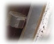
Why worry? Tapered tires cause the trunnions to wear or adjust in a "dovetail" fashion which causes extreme thrust, wear, amperage problems and trunnion and idler bearing failures.
